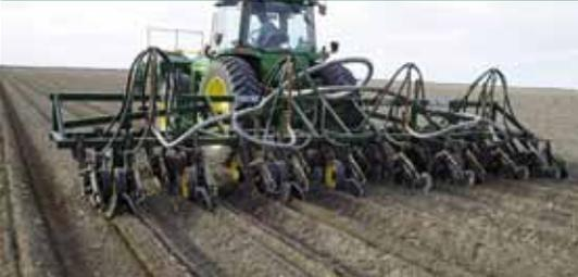
Ideal for seeding, fertilising and gassing into heavy trash cover and clayish, sticky soils. Excellent ground penetration in tight soils. Frames to suit 9", 10", 12", 13" and 15" row spacings. Easy access to row units.
