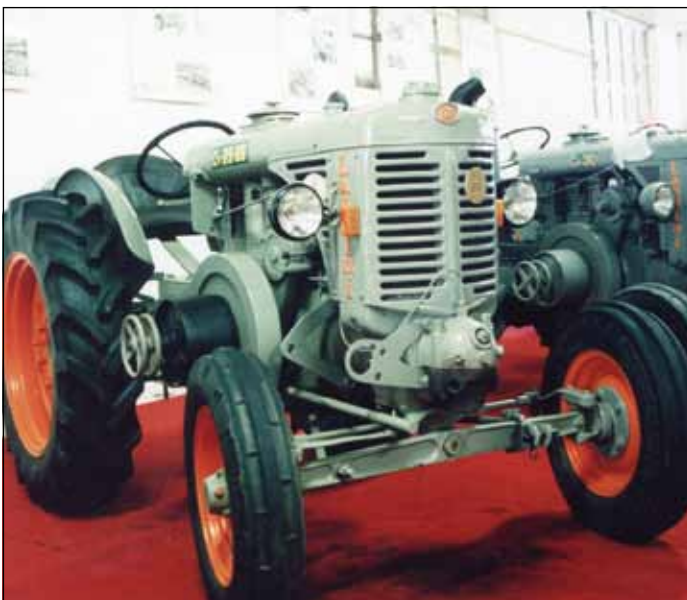
The Cv 25-30, produced in the early 1950s was equipped with 3 point linkage and sold strongly to small acre farmers in various parts of the world. The unit pictured is on display in the Fabbrico Landini Museum. (Photo IMJ)
